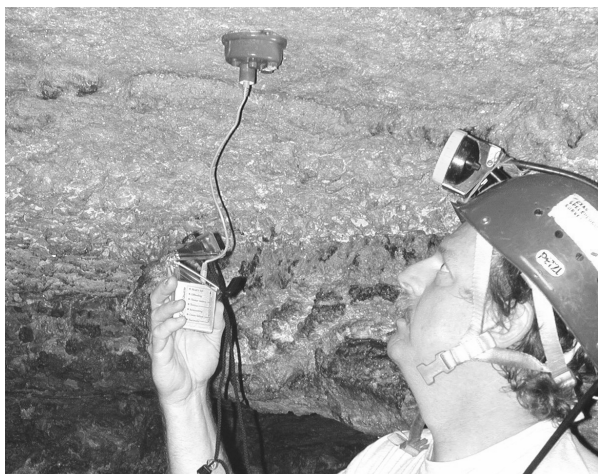
Figure 1. William R. Elliott uses an Onset Hobo® Data Shuttle to offload temperature and humidity data from the Hobo® H8 Pro data logger. The shuttle can hold data from up to seven data loggers.
